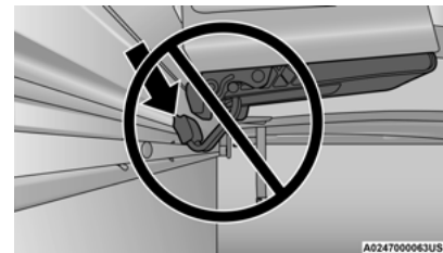
Improper Clamp Position
