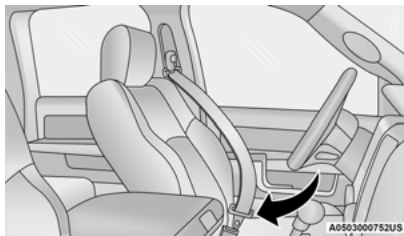
Inserting Latch Plate Into Buckle
