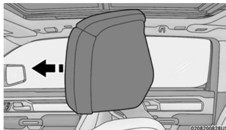
Forward Adjustment (Power Head Restraint)
