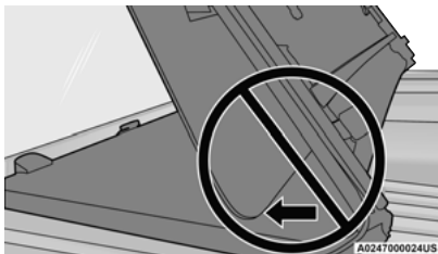
Incorrect Folding — Will Cause Damage
