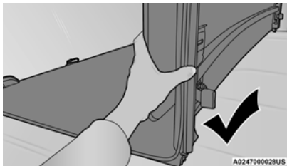
Correct Folding — Hold Panels Together
