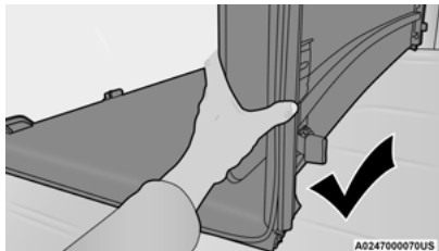
Correct Folding — Hold Panels Together
