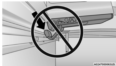
Improper Clamp Position
