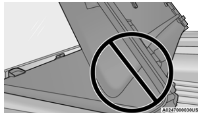
Incorrect Folding – Will Cause Damage
