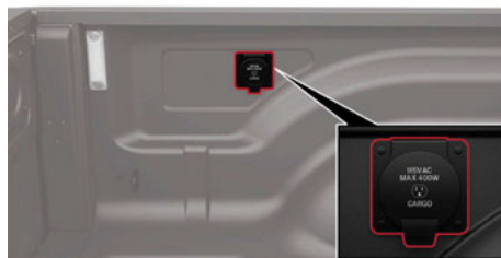
Exterior Power Inverter (If Equipped)
