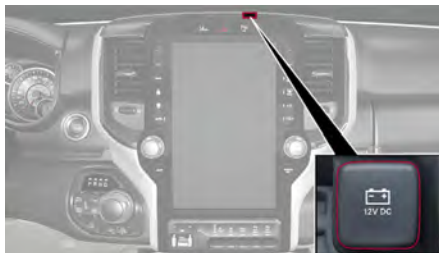
Power Outlet — Top Of Center Stack
