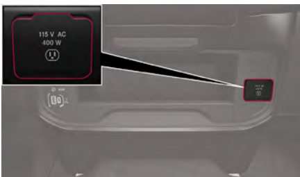
Center Stack Power Inverter Outlet
