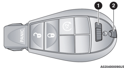
Emergency Key Removal (Standard Ignition Key Fob)
