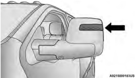
Forward Utility Light
