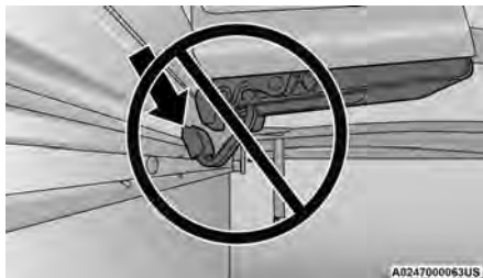
Improper Clamp Position
