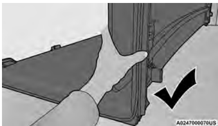
Correct Folding – Hold Panels Together
