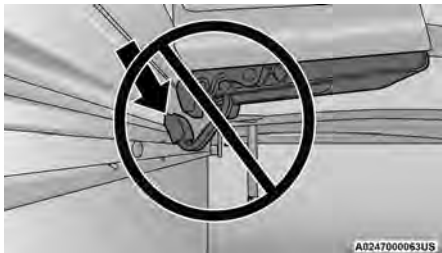
Improper Clamp Position
