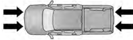
Jack / Extensions Placement
