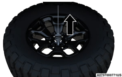
Pulling The Retainer Through The Center Of The Wheel
