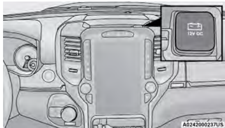
Power Outlet – Top Of Center Stack
