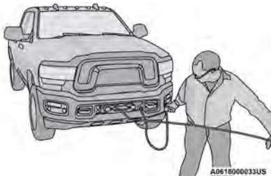
Pulling Synthetic Rope Under Tension
