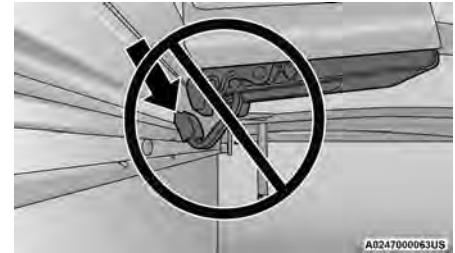
Improper Clamp Position
