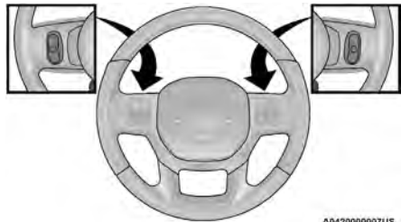
Remote Sound System Controls
