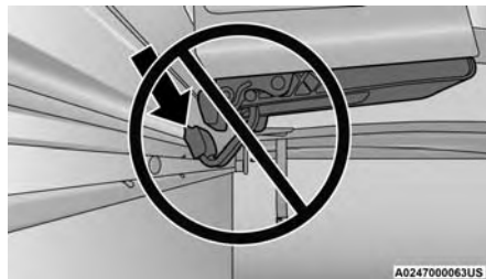
Improper Clamp Position
