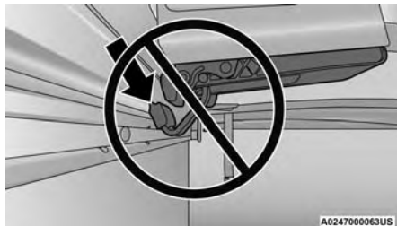
Improper Clamp Position
