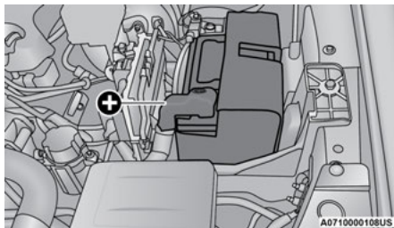
Positive (+) Battery Post
