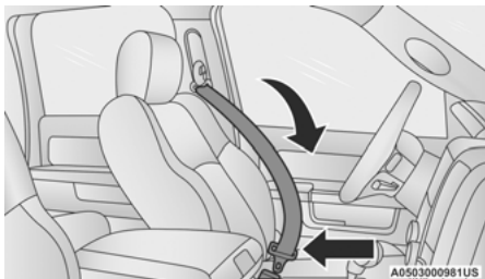
Pulling Out The Latch Plate
