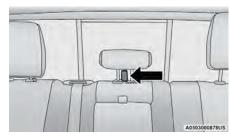
Tether Strap Loop With Center Head Restraint In Raised
