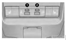
Rear Center Console Standard (Type A) USB Ports
