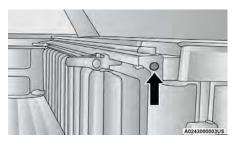
**End Cap Screw Location If Equipped With Tonneau Cover**
