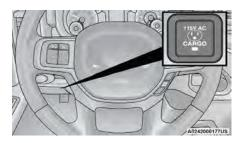
Instrument Panel Power Inverter Switch
