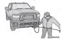
**Pulling Synthetic Rope Under Tension**
