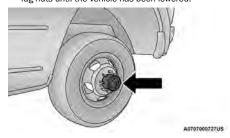
Rear Inner Wheel Proper Placement (Dual Rear Wheel Equipped)
