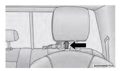
Tether Strap Through Outboard Tether Strap Loop
