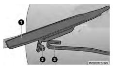
**Removing Wiper From Wiper Arm**
