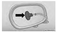
**Removing Bulb Socket From Clearance Lamp**
