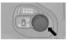
**Electronic Transmission Gear Selector**
