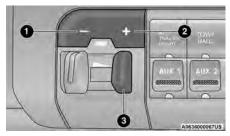
Integrated Trailer Brake Module (ITBM)
