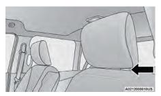
**Head Restraint Adjustment Button Location**
