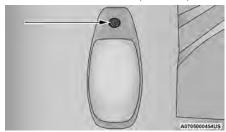
**Removing Rear Screw From Clearance Lamp**
