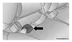
Mini-Latch And Mini-Buckle Connected
