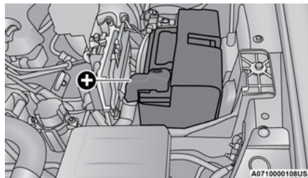
Positive Battery Post
