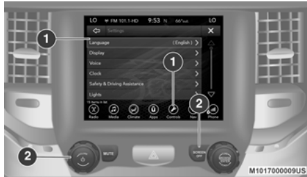
Uconnect 4/4C/4C NAV With 8.4-inch Display Buttons On The Touchscreen And Buttons On The Faceplate
