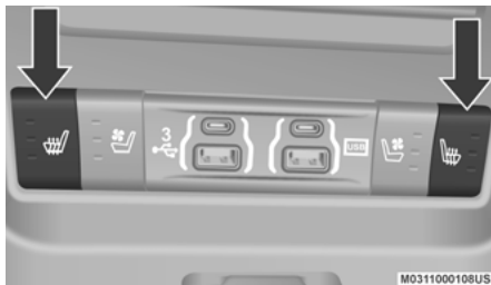
Rear Heated Seat Switches
