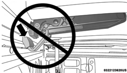
Improper Clamp Position
