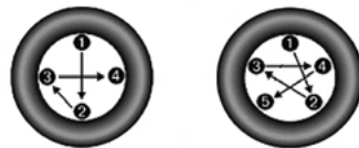
Four And Five Lug Nuts/Bolts Torque Pattern
