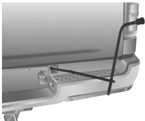
Inserting The Extension Tubes Into The Access Hole
