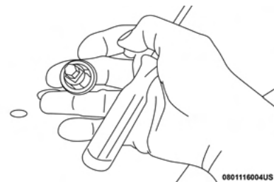
Removing The Bulb From The Bulb Socket
