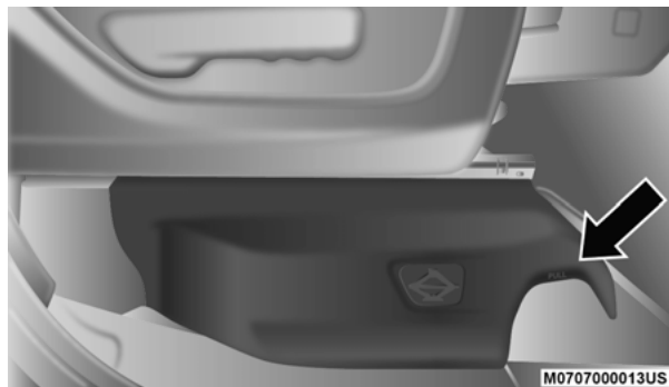
Pull Jack Access Cover From Front
