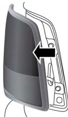
Pulling Out The Tail Lamp
