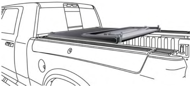
Intermediate Position (Vehicle Cannot Be Driven)
