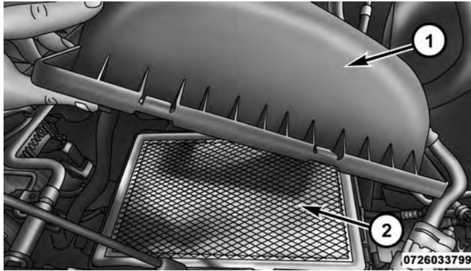
Open Air Cleaner Filter Assembly
