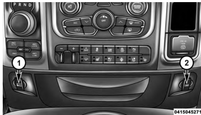
Power Outlets — Center Stack
