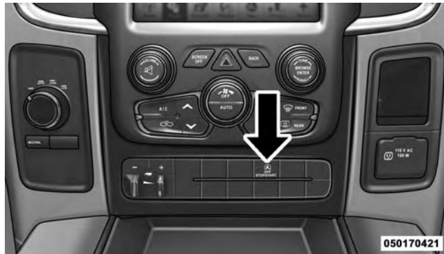
STOP/START OFF Switch
