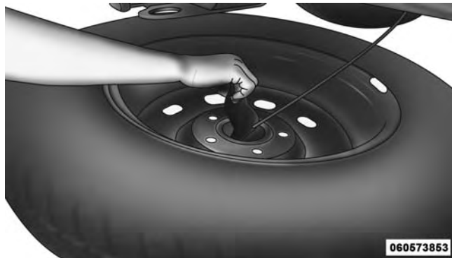
Reinstalling The Retainer
