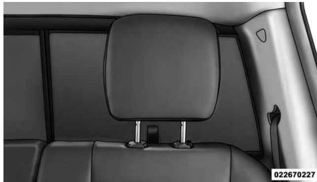
Head Restraint In Raised Position
