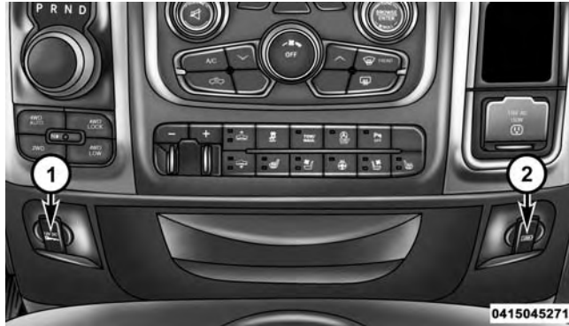
Power Outlets — Center Stack
