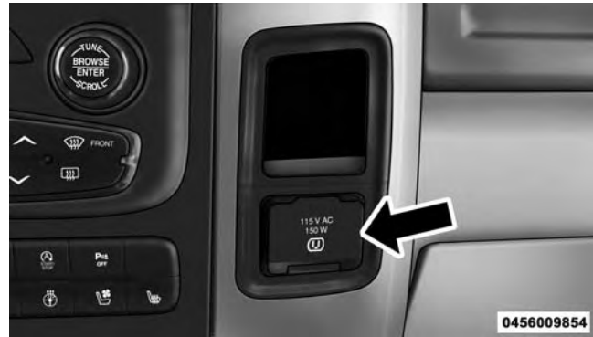
Power Inverter Outlet
