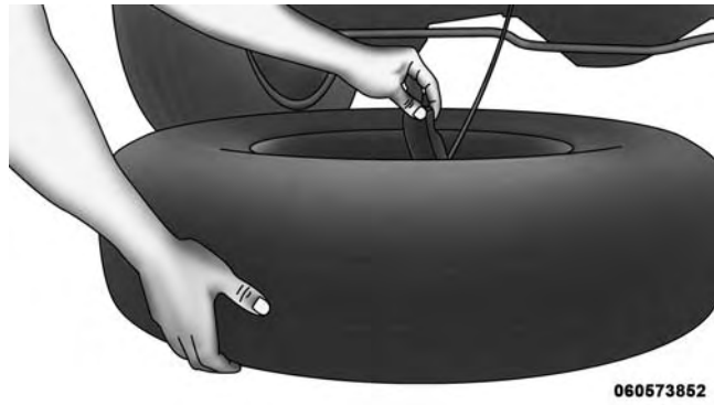
Gaining Access To The Retainer
