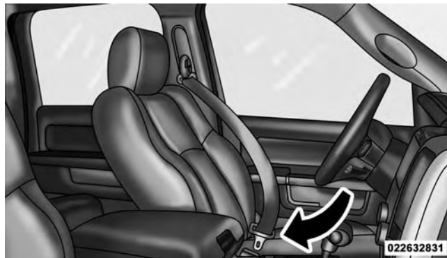
Inserting Latch Plate Into Buckle
