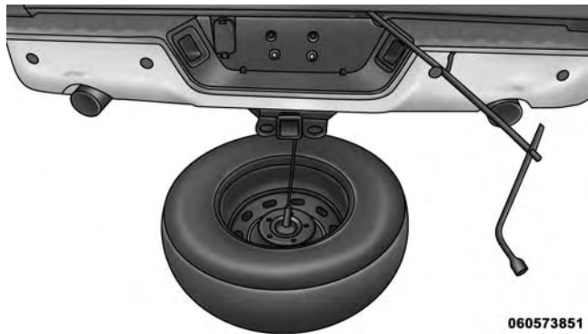
Pulling The Spare Tire Out
