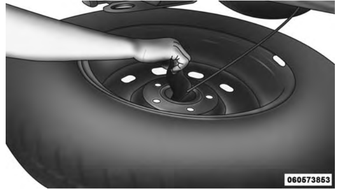
Reinstalling The Retainer
