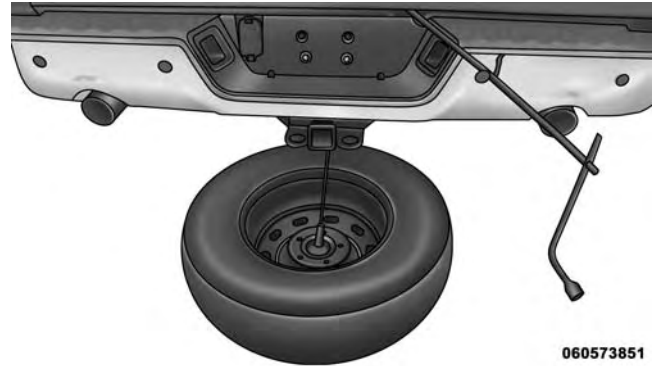
Pulling The Spare Tire Out
