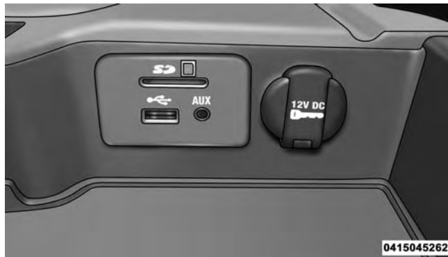
Power Outlet — Upper Lid
