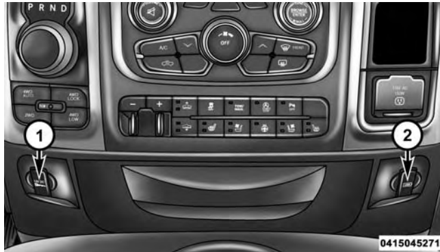
Power Outlets — Center Stack
