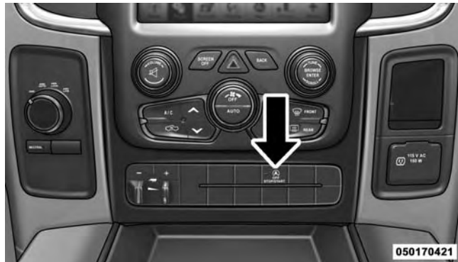
STOP/START OFF Switch
