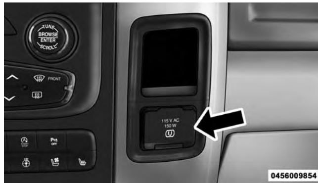
Power Inverter Outlet
