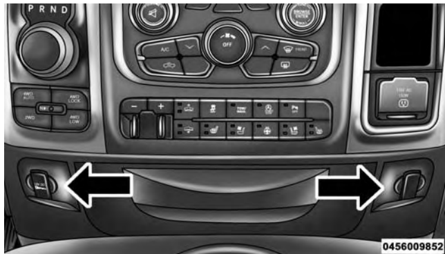
Power Outlets — Center Stack
