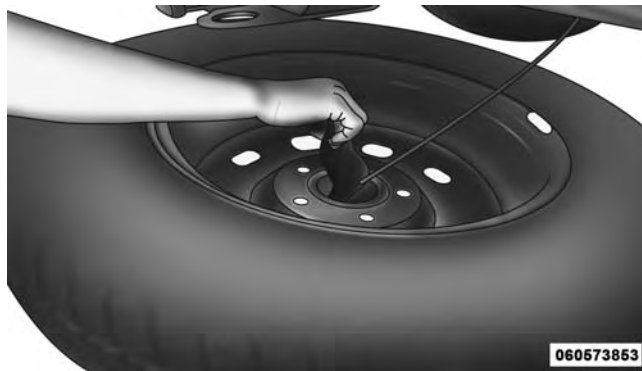
Reinstalling The Retainer
