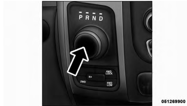
Electronic Transmission Shifter
