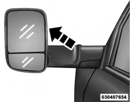
Trailer Towing Position
