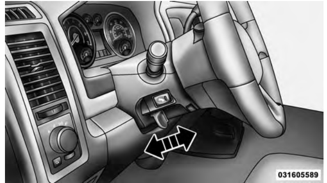
Tilt Steering Lever
