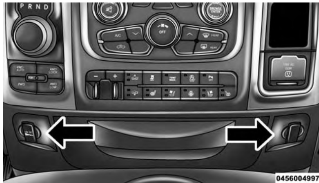
Power Outlets — Center Stack
