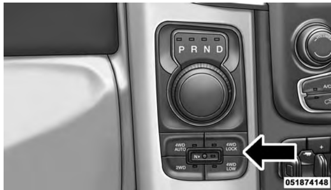
Transfer Case Switch (Five-Position)
