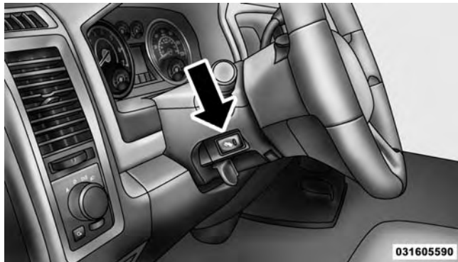
Adjustable Pedals Switch
