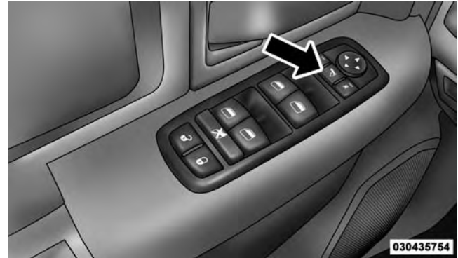
Power Folding Mirror Switch
