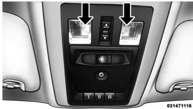
Front Courtesy/Reading Lights
