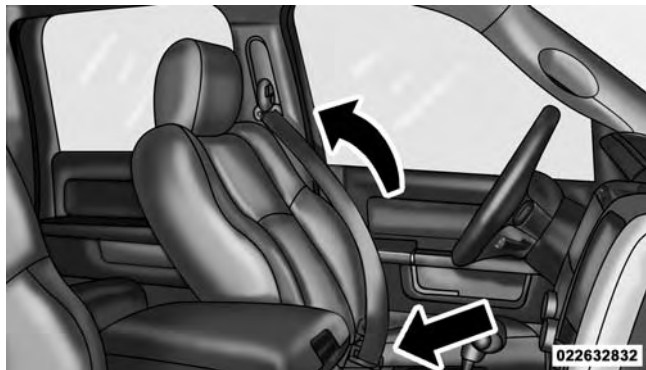
Removing Slack From Belt
