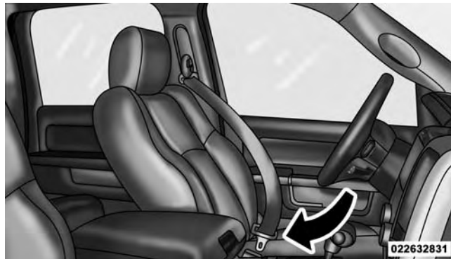
Latch Plate To Buckle
