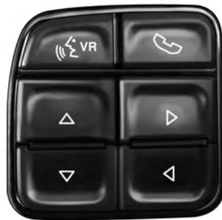
EVIC Steering Wheels Buttons
