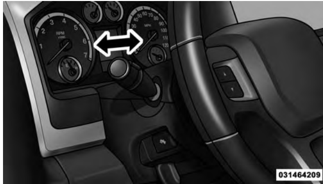
High/Low Beam Switch
