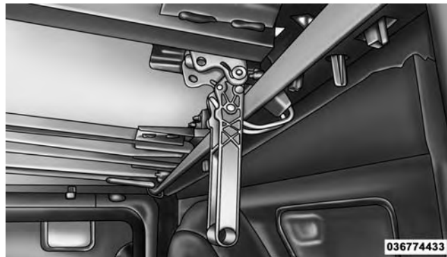
Semi Clamped Position
