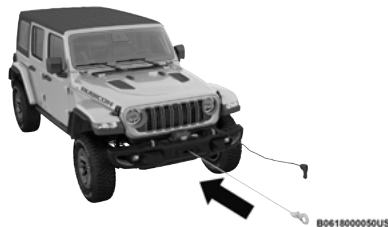
Rewinding The Synthetic Rope
