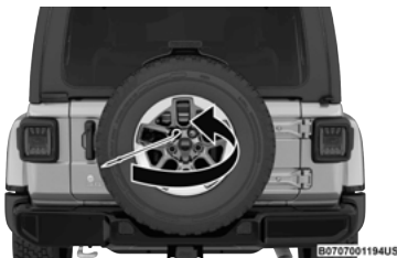
Removing The Spare Tire
