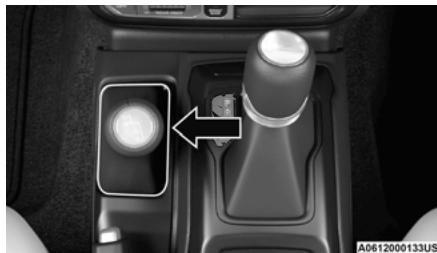
Four-Wheel Drive Gear Selector
