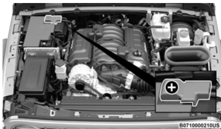
Positive (+) Battery Post (6.4 Engine)
