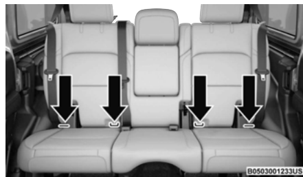
LATCH Anchorages (Four-Door Models)
