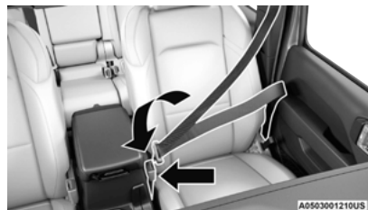
Inserting Latch Plate Into Buckle
