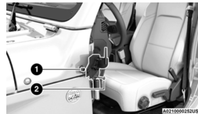
Attaching Mirror Bracket To The Vehicle
