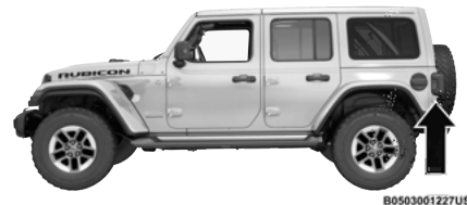
BSM Radar Location (Left Side Shown)
