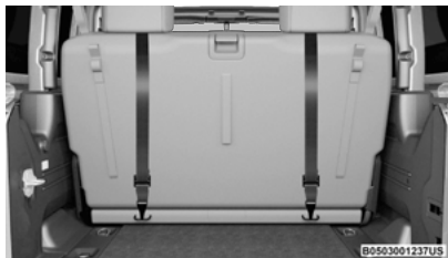
Tether Strap Mounting (Two-Door Models)
