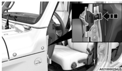
Push Bracket Onto A-pillar
