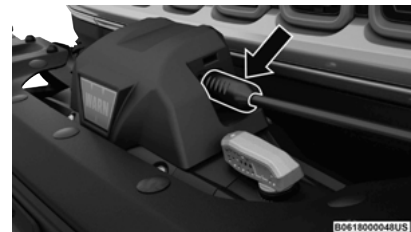
Winch Box Remote Control Connector
