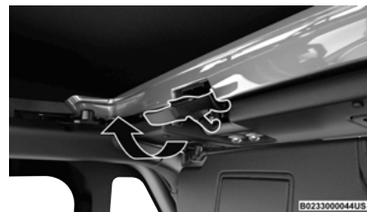
Engage Both Header Latches
