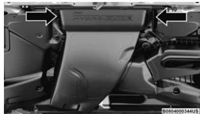
First Water Chamber Removal
