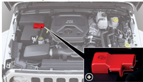
Positive (+) Battery Post Location
