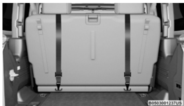
Tether Strap Mounting (Two-Door Models)
