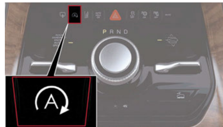
Stop/Start OFF Switch
