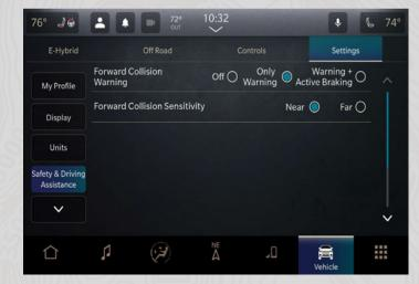
The system can be turned on or off through your touchscreen. You can also use your touchscreen to adjust the system's sensitivity and active braking status.
