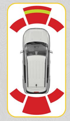
When the sensors detect an obstacle, a chime will sound and the ParkSense Park Assist warning will appear in the instrument cluster display. The system will show arcs in the area of the obstacle based on relative distance and location. As you approach the obstacle, the arcs will move and the chime will change from slow to fast to continuous.
