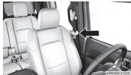
Pulling Out The Latch Plate
