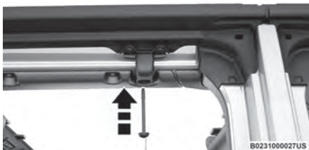
Insert Screws From Below Frame
