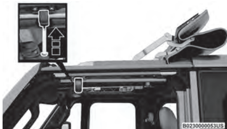
Attach Front Door Rail Bolt
