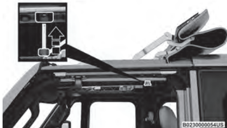
Attach Rear Door Rail Bolt
