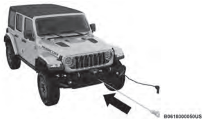
Rewinding The Synthetic Rope
