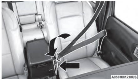
Inserting Latch Plate Into Buckle
