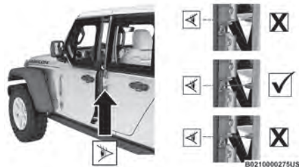
Check Door Latch And Striker Alignment
