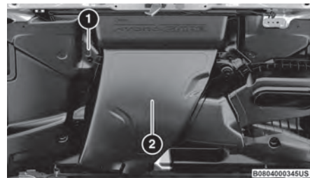
First Water Separation Chamber
