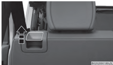
Lift Seatback Release Lever Up
