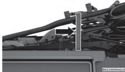
Hook-And-Loop Fastener Placement
