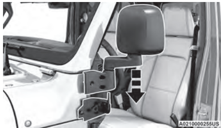
Lower Mirror Assembly Onto Bracket
