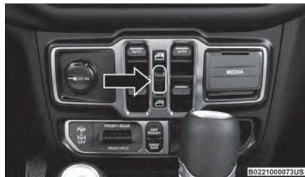
Window Lockout Switch
