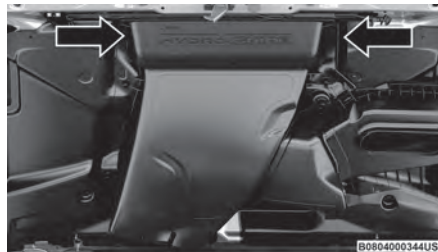
First Water Chamber Removal
