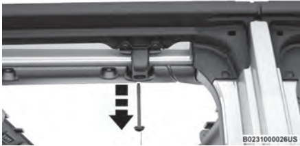
Remove Screws From Below Frame
