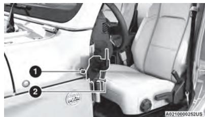
Attaching Mirror Bracket To The Vehicle
