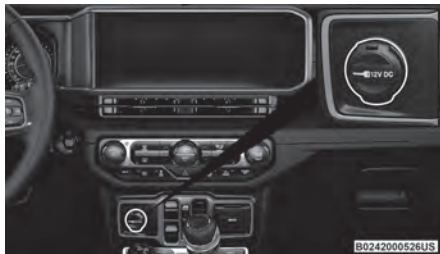
Front Power Outlet
