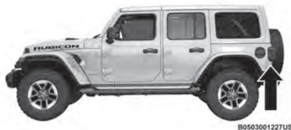
BSM Radar Location (Left Side Shown)
