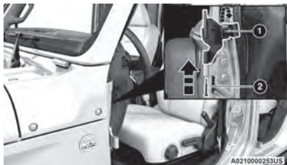
Attaching Mirror Bracket To The Vehicle
