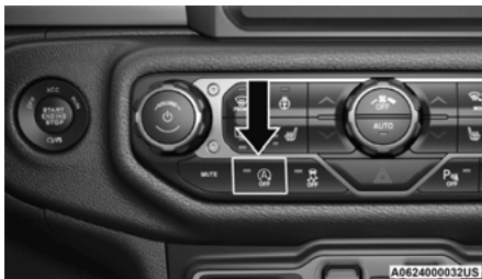
Stop/Start OFF Switch
