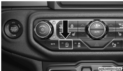
Stop/Start OFF Switch
