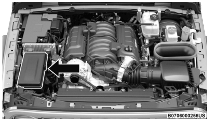
Power Distribution Center Location (6.4 Engine)
