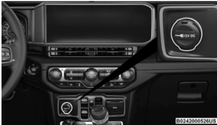
Front Power Outlet
