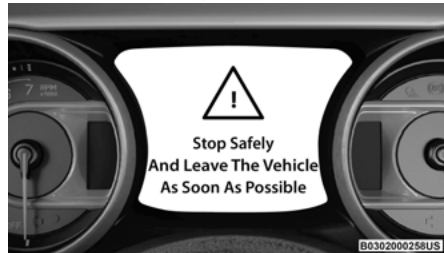
Stop Safely And Leave The Vehicle As Soon As Possible Warning Message
