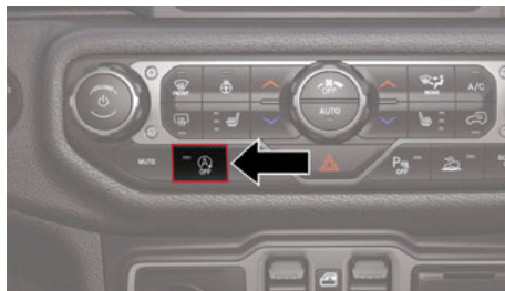
Stop/Start OFF Switch
