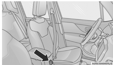
Inserting Latch Plate Into Buckle
