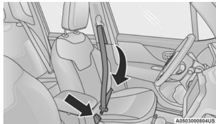
Pulling Out The Latch Plate
