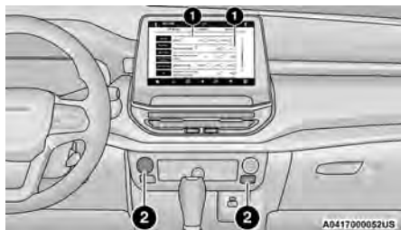
Uconnect 5/5 NAV With 10.1-inch Display Buttons On The Faceplate And Buttons On The Touchscreen
