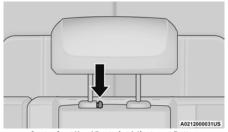
**Center Seat Head Restraint Adjustment Button**
