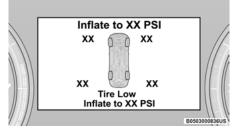
**Low Tire Pressure Monitoring System Display**
