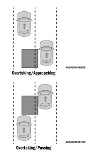
The BSM system is designed not to issue an alert on stationary objects such as guardrails, posts, walls, foliage, berms, etc. However, occasionally the system may alert on such objects. This is normal operation and your vehicle does not require service.
