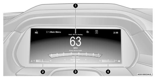
Holding the **OK** button on the Instrument Cluster Display controls located on the steering wheel will allow you to change your display from Digital to Analog.
