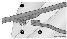
**Wiper Blade Removed From Wiper Arm**
