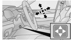
Power Tilt/Telescoping Steering Control Location
