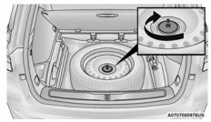
Reinstalling Tire Fastener
