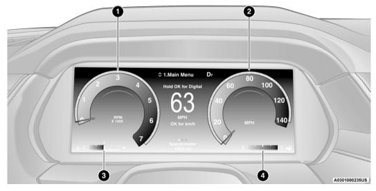
Holding the OK button on the Instrument Cluster Display controls located on the steering wheel will allow you to change your display from Analog to Digital.
