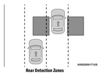
When the vehicle is started, the BSM Warning Light will momentarily illuminate in both outside rearview mirrors to let the driver know that the system is operational. The BSM system sensors operate when the vehicle is in any forward gear.
