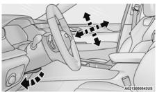
Manual Tilt/Telescoping Steering Column Handle
