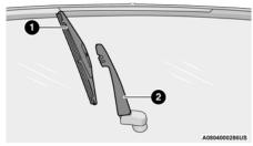
Wiper Blade Removed From Wiper Arm
