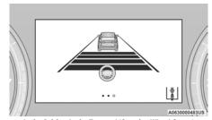
Active Driving Assist Engaged (Steering Wheel Green)
