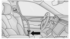
**Inserting Latch Plate Into Buckle**
