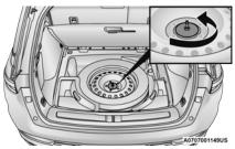
**Removing The Spare Tire Fastener**
