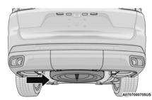
**Road Wheel Installed In Spare Location**
