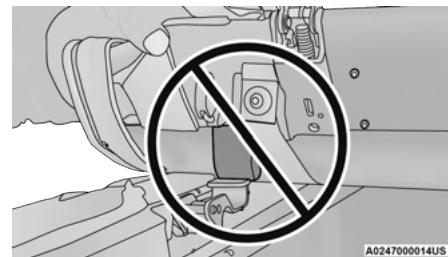
Incorrectly Seated Retainer
