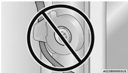
Incorrectly Seated Tailgate Strap
