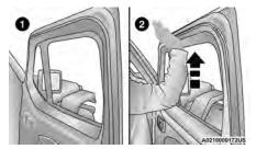
**Push Upward To Remove Upper Half-Door**
