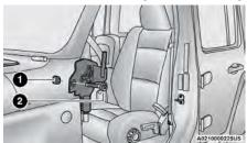
**Attaching Mirror Bracket To The Vehicle**
