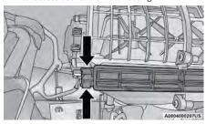
**Air Filter Retaining Tabs**
