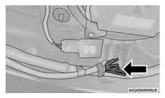
**Auxiliary Switch Connections - Under Instrument Panel**
