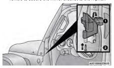
**Attaching Mirror Bracket To The Vehicle**
