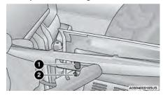
**Wiper Blade Removed From Wiper Arm**
