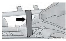
**Hook-And-Loop Fastener Placement**
