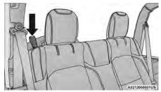
**Rear Head Restraint Folding Strap Location**
