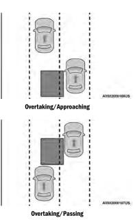
The BSM system is designed not to issue an alert on stationary objects such as guardrails, posts, walls, foliage, berms, etc. However, occasionally the system may alert on such objects. This is normal operation and your vehicle does not require service.
