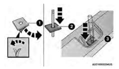
**Press Shim Firmly Into Bottom Of Pocket**
