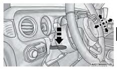
Tilt/Telescoping Steering Column Lever
