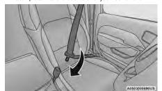
**Inserting Latch Plate Into Buckle**
