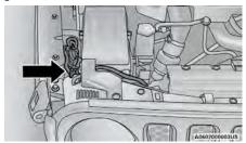
**Diesel Engine Block Heater Cord Location**
