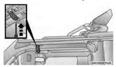
**Attach Front Door Rail Bolt**
