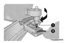
**Rotate Screw For Seal Compression**
