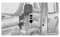
**Lower Mirror Assembly Onto Bracket**
