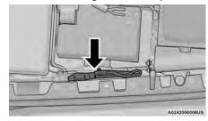
**Auxiliary Switch Connections - Under Hood**
