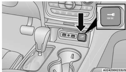
Front Power Outlet
