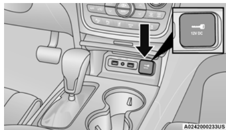
Front Power Outlet
