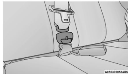
Inserting Mini-Latch Plate Into Mini-Buckle
