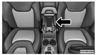
**Upper Console Charging Pad**To open, pull up on the latch and lift the cover.
