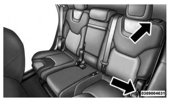
Rear Seatback Release Lever And Pull Strap
