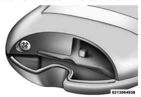
Remove Screw From Transmitter Case
