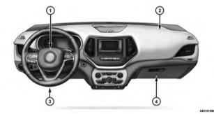
1 — Driver Advanced Front Air 3 — Supplemental Driver Side Bag 2 — Passenger Advanced Front Air Bag
