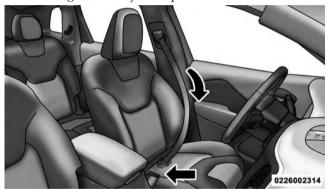
Pulling Out The Lap/Shoulder Belt Latch Plate
