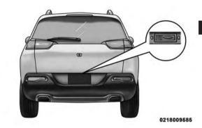
Electronic Liftgate Release/Liftgate Passive Entry Location
