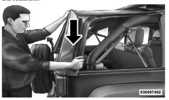
12. To install the side windows, affix the window temporarily by attaching it to the Velcro® in the upper rear corner. Start the zipper but close only about 1 in (2.5 cm).
