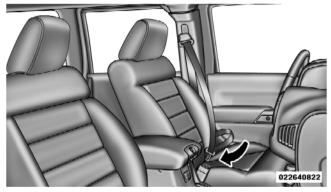
**Inserting Latch Plate Into Buckle**
