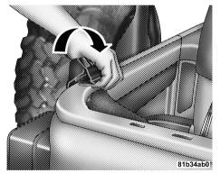
14. Completely release the latches from the loops on the windshield frame. If your vehicle is not equipped with the Sunrider® package, proceed to Step 15.
