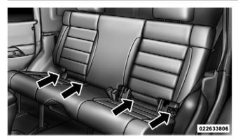
**Latch Anchorages (Four-Door Models)** In addition, there are tether strap anchorages behind each rear seating position located on the back of the seat.
