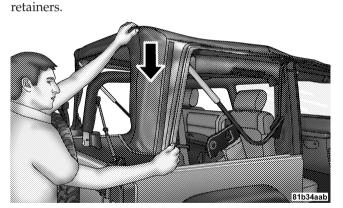
10. To install the side windows, affix the window temporarily by attaching to the Velcro® in the rear corner. Start the zipper but close only about 1 in (2.5 cm).
