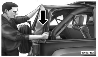
3. Rotate the header forward.
