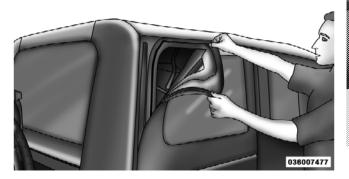
2. Release header latches from the windshield frame.
