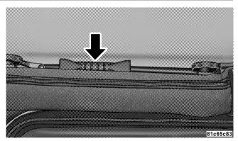
4. Grasp the header and lift the top back. Make sure the material is folded back as shown.
