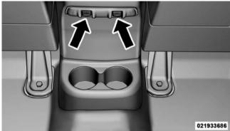
Rear Power Window Switches (Four-Door Models) Wind Buffeting
