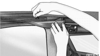
11. Insert the front retainer of the window into the door channel, making sure the retainer is fully seated and properly positioned on the door frame. Failure to do so can result in wind and water leaks or damage to the window.
