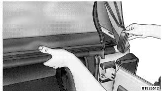
17. Insert the rear window retainer into the swing gate bracket on both the left and right sides.
