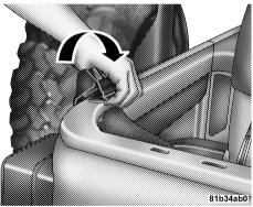
13. The swing gate brackets do not need to be removed 14. Grasp the front side bow behind the header, and lift unless the hard top is being installed. To remove the the top.
