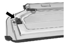
**NOTE:** The front panel(s) must be positioned properly to ensure sealing. Set the panels on the windshield frame so that there is no overhang. Also, make sure that the panels are sitting flush with the body.
