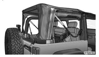
9. Partially install the sail panel retainers into the body side channel, leaving the last 3 in (7.6 cm) toward the rear window loose (on both sides). Pulling down on the rear roof bow (3–bow) will aid to reach the channel with the
