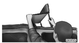
5. Locate the straps to secure the side bows. Wrap the straps around the bows as shown. Repeat on the other side.
