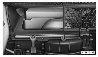
6. Remove the two particulate air filters from the HVAC air inlet housing. Pull the filter elements straight out of the housing, one at a time.
