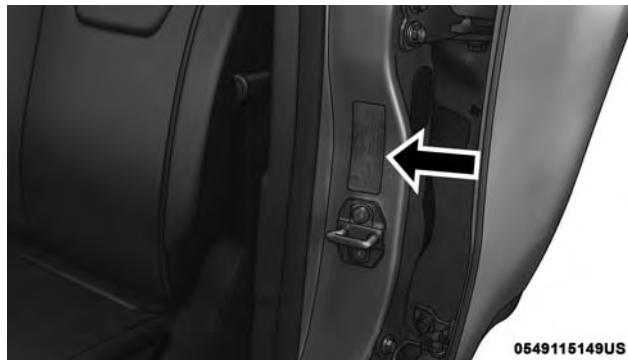
Example Tire Placard Location (B-Pillar)
