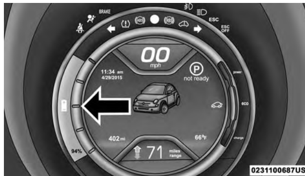
High Voltage Battery Gauge
