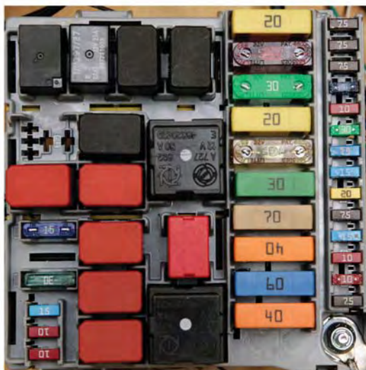
F15 Fuse 15 Amp Blue - Cigar Lighter/Power Outlet Front Console
