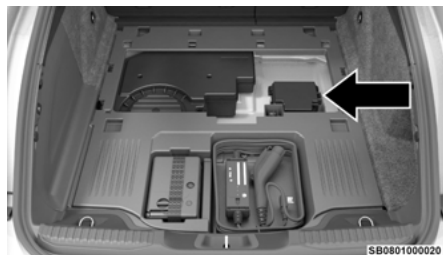
Rear Power Distribution Center
