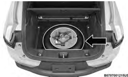
Damaged Tire Storage
