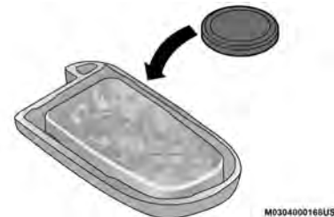
Key Fob Battery Replacement
