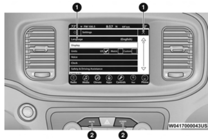
Uconnect 4C/4C NAV With 8.4-inch Display Buttons On The Faceplate And Buttons On The Touchscreen
