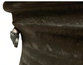
Incorrect Wheel Rim Contact
