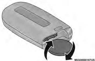
Separating Case With A Coin
