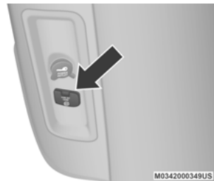
Power Inverter Outlet
