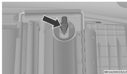
Storage Bin Cover Emergency Release Lever
