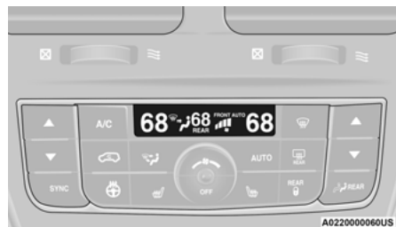
Automatic Temperature Controls
