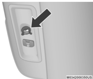
Rear Panel Power Outlet
