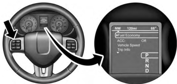
Electronic Vehicle Information Center (EVIC)
