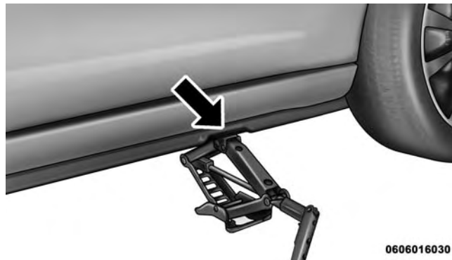
Jack Engaged (Rear Jacking Location)
